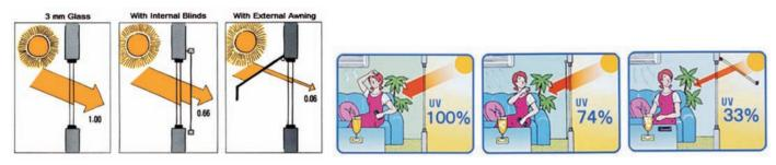
According to research done by the Awning Association of Japan, external awnings reduce UV penetration by as much as 75% and lower the indoor temperature by 8-15degrees.
